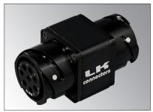
The **LKI 08 adapter** features a male and female LKI 08 connector mounted back to back without locking rings. It enables the connection of two 8 pin extension cables, thus obtaining the desired length needed.
