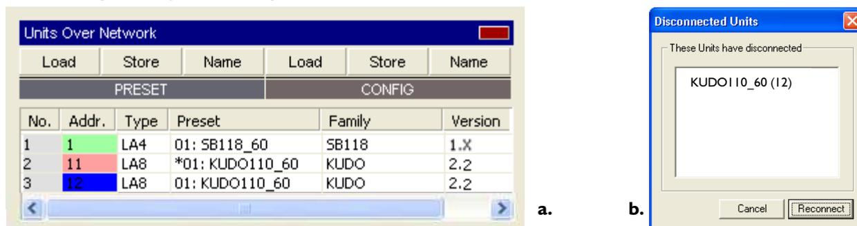
Figure 16: (a) Units Over Network window (b) Disconnected Units window
