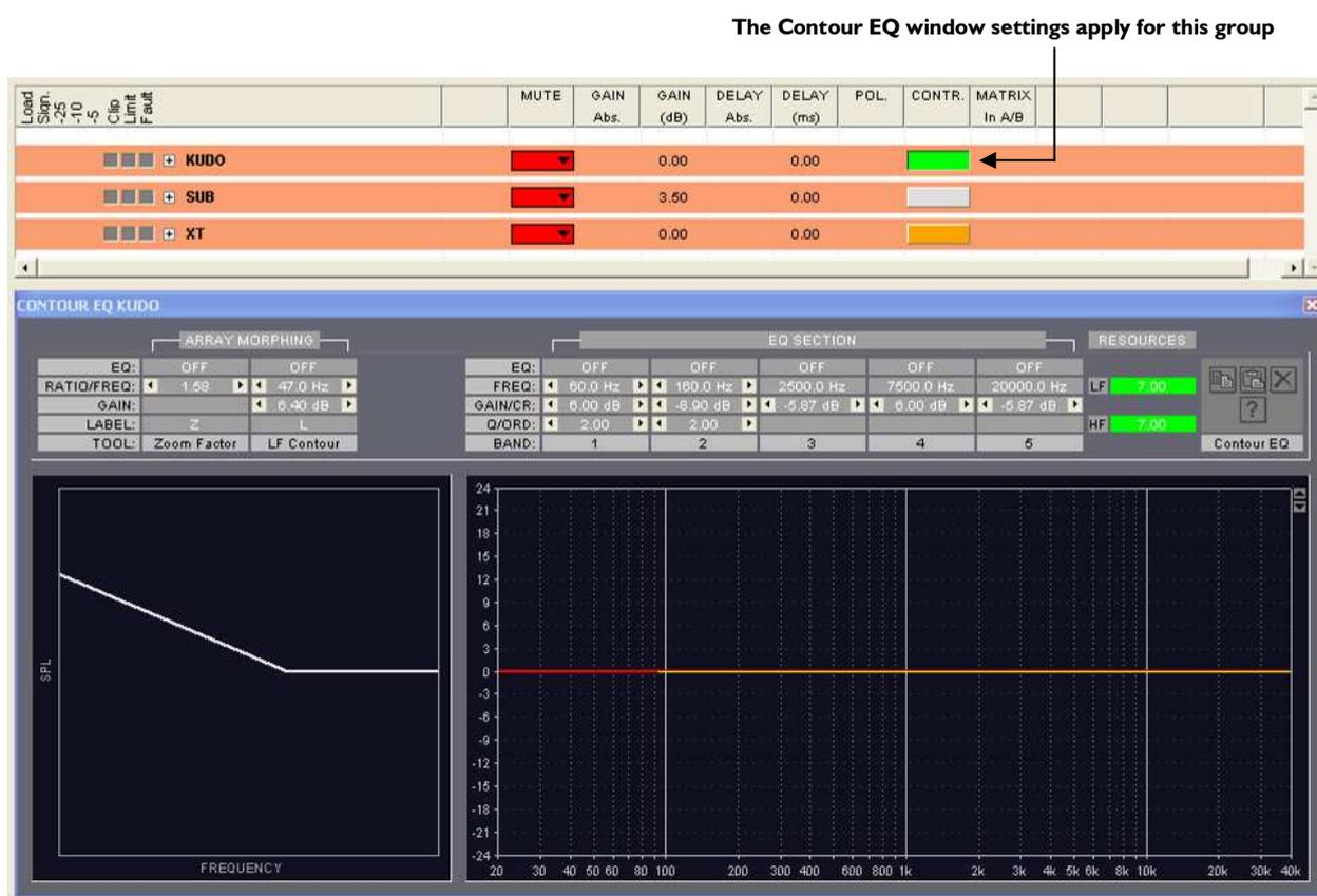
Figure 25: Displaying the **Contour EQ** window for the **KUDO** group
